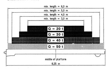
Load gravity center must be inside the rispective marked areas
